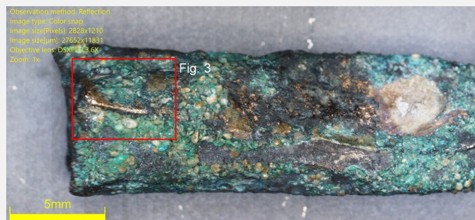
Fig. 2: Lake (shiny brown) and terrestrial (granulated green-blue) crust of the Tang with lacuna showing the underlying metal and detail of Fig. 3,
