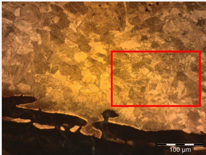
Fig. 8: Micrograph of the metal structure from Fig. 7 (detail), etched, bright field, 50x. The alpha phase of the alloy shows polygonal grains. Area of Fig. 9 is marked by a red rectangle,
