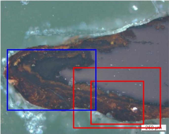
Fig. 12: Micrograph showing the metal - corrosion crust interface from Fig. 3 (detail) unetched, polarised light. The micrographs of Fig. 11 and Fig. 13 are marked by the large and small red rectangles respectively while the area selected for elemental chemical distribution (Fig. 14) is marked by the blue rectangle. The light-grey layer of Fig. 11 (arrow) appears black whereas the rest of the corrosion layer is brown, red and orange,
