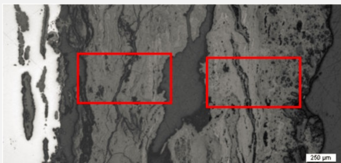
Fig. 11: Micrograph showing the metal - corrosion crust interface from Fig. 3 (reversed picture, detail), unetched, bright field. The areas selected for elemental chemical distributions (Fig. 13 (left) and Fig. 14 (right)) are marked by red rectangles,
