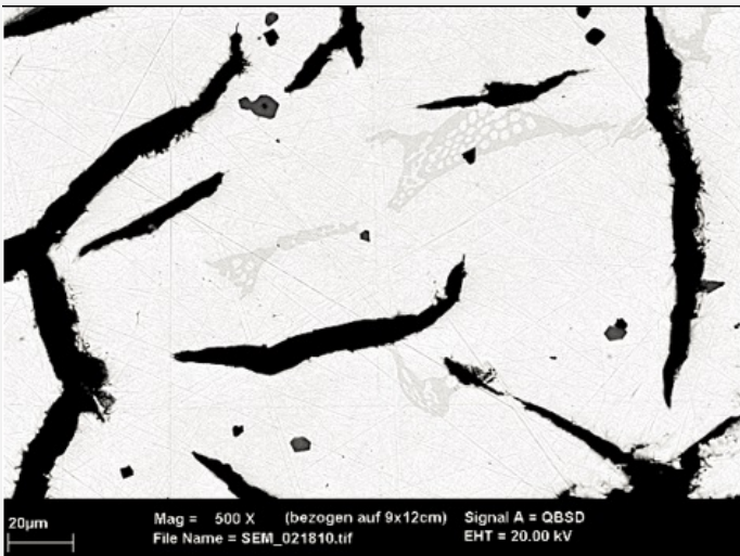
Fig. 6: SEM image from Fig. 3 (detail), BSE-mode, unetched. We observe the graphite flakes in black, the manganese sulphide inclusions in grey and the eutectic mixture in light-grey,
