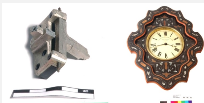
Fig. 1: Broken armature (left) from the clock movement of a wooden wall clock (right) (after Seematter 2009),
