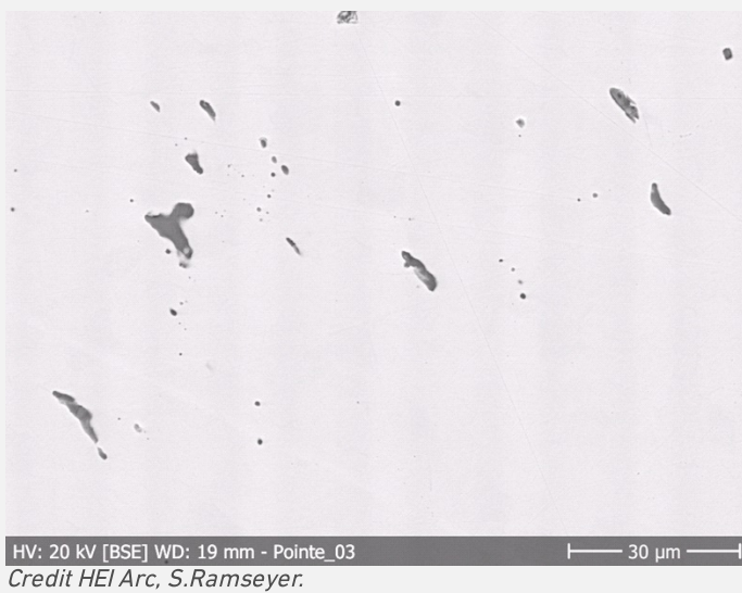
Fig. 8: SEM, BSE-mode picture of inclusions in remaining metal,
