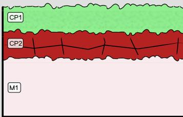
Fig. 9: Stratigraphic representation of the axe (sample 3) under binocular using the MiCorr application. The characteristics of the strata are only accessible by clicking on the drawing that redirects you to the search tool by stratigraphy representation. This presentation can be compared to Fig. 18. CP1 corresponds to CP1c, Credit HE-Arc CR, C.Degrigny.
