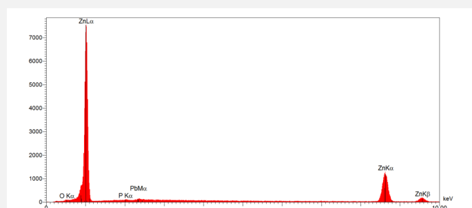
Fig. 6: Chemical composition of the metal. Method of analysis: SEM-EDS. Lab. of Electronic Microscopy and Microanalysis, Néode, HEI Arc,
