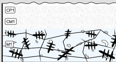
Fig. 6: Stratigraphic representation of the sample taken from the domed cap nut in cross-section (DF) using the MiCorr application. The characteristics of the strata are only accessible by clicking on the drawing that redirects you to the search tool by stratigraphy representation. Area where the metal plating is missing. CP1 corresponds to CP2 in Fig. 3, CM1 represents the corroded metal phase, while M1 corresponds to the bulk metal (M2 in Fig. 3 and Fig. 5), Credit UiO-IAKH, M.Hovind.
