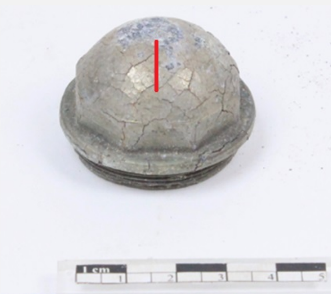
Fig. 2: Zone of the artefact submitted to visual observation and location of sampling area (a cross-section of the metal marked by the red line),
