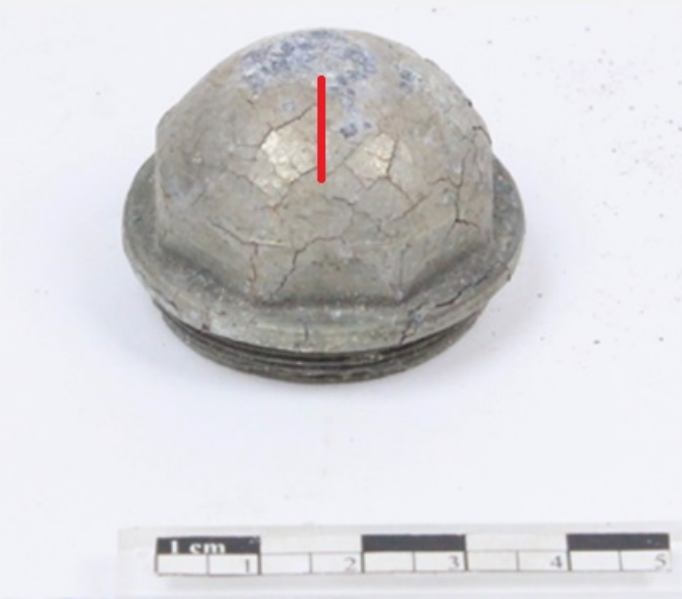
Fig. 2: Zone of the artefact submitted to visual observation and location of sampling area (a cross-section of the metal marked by the red line),
