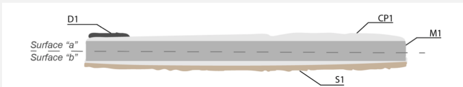
Fig. 3: Schematic presentation of the artefact based on visual macroscopic observation. CP = corrosion product, D = deposit, M = metal, S = soil,
