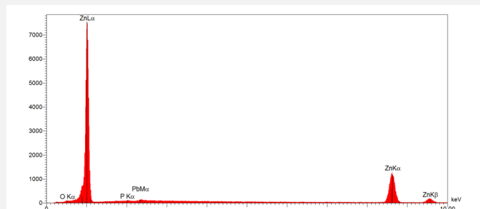
Fig. 5: Chemical composition of the metal. Method of analysis: SEM-EDS. Lab. of Electronic Microscopy and Microanalysis, Néode, HEI Arc,
