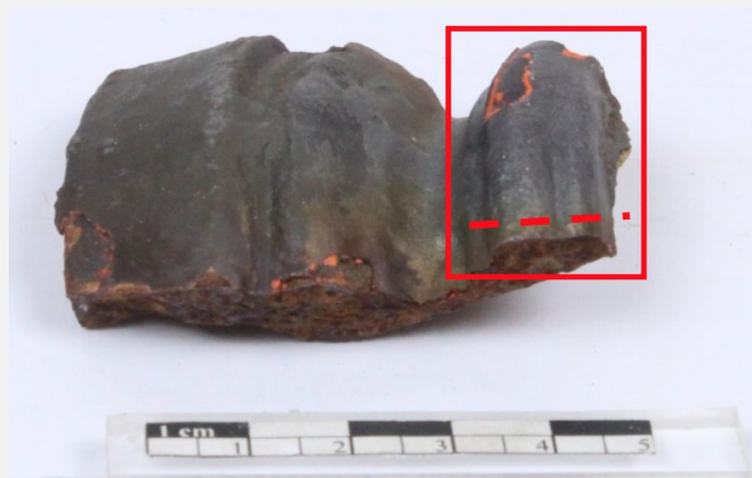
Fig. 2: Zone of the artefact submitted to visual observation (red square) and location of sampling (a cross section through metal including a few layers of paint, marked by the stippled line),
