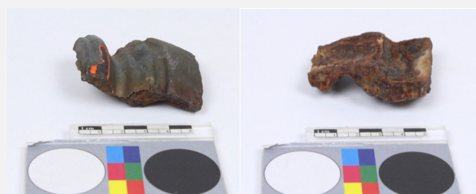
Fig. 1: Lamp post (?) fragment with paint coating; exterior (coated) surface and the rear (non-coated) surface to the left and right, respectively,
