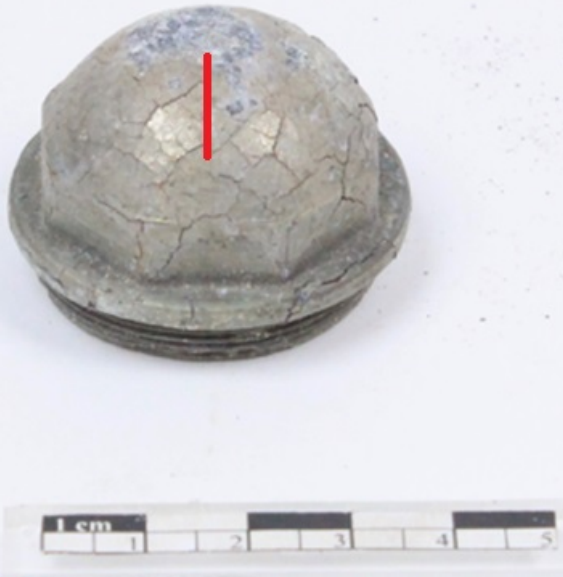
Fig. 2: Zone of the artefact submitted to visual observation and location of sampling area (a cross-section of the metal marked by the red line),
