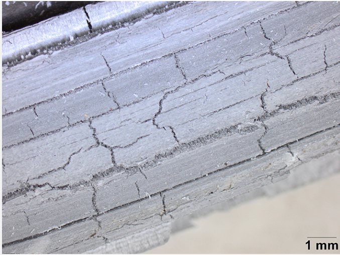
Fig. 3: Detail of the corroded lead came,
