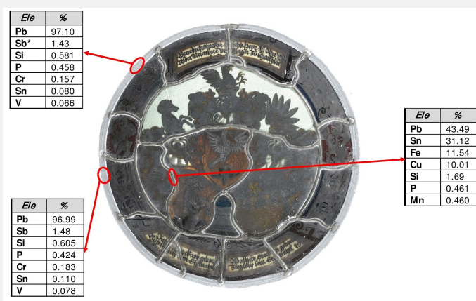
Fig. 6: XRF analyses of a selection of the comes,
