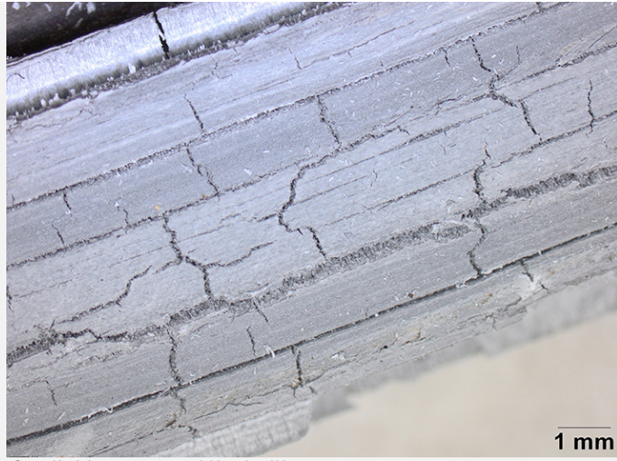
Fig. 3: Detail of the corroded lead came,
