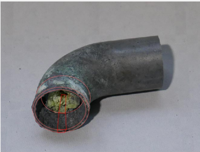
Fig. 3: Heavily corroded side of the Bugatti water pipe showing the sampling area indicated in red,
