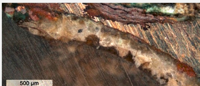
Fig. 11: Micrograph of the metal sample (area 2) from Fig.8 (detail) and corresponding to the stratigraphy of Fig. 13, dark field,
