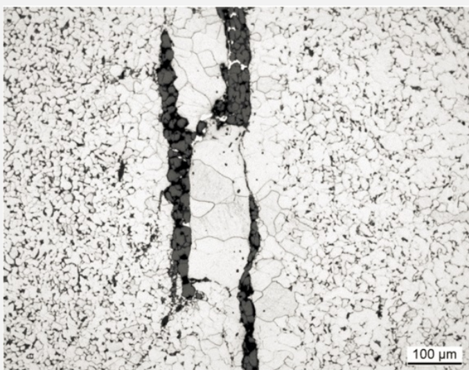
Fig. 8: Micrograph of metal sample 2 from Fig. 3 (detail), nital etched, bright field. We observe a hypoeutectoid steel including a ferritic zone surrounded by slag inclusions,
