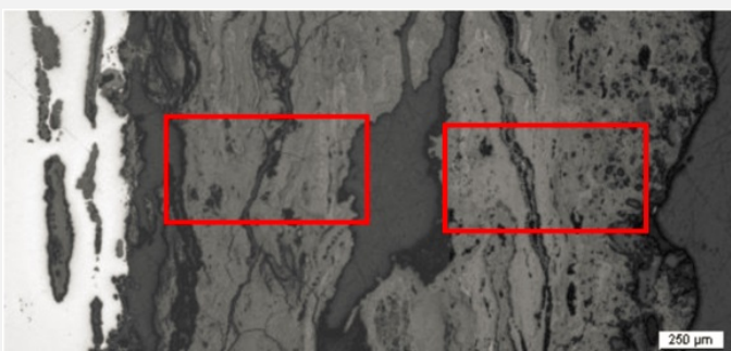
Fig. 10: Micrograph showing the metal - corrosion crust interface from Fig. 3 (reversed picture, detail), unetched, bright field. The areas selected for elemental chemical distributions (Fig. 12 (left) and Fig. 13 (right)) are marked by red rectangles,
