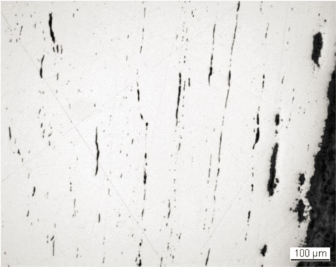
Fig. 4: Micrograph of metal sample 1 from Fig. 3 (reversed picture, detail), unetched, bright field. Slag inclusions organized in rows mark the welding seams,
