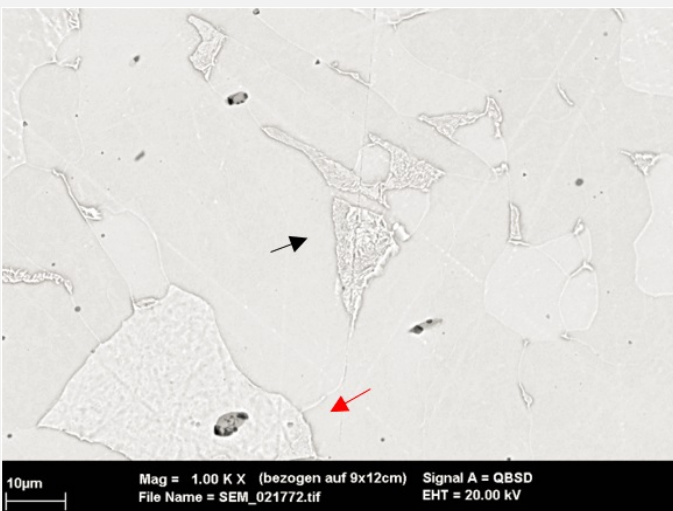
Fig. 7: SEM image of the metal sample from Fig. 3 (detail), BSE-mode, nital etched, bright field. The white ferrite grains contain lamellar pearlite (black arrow) and lenticular grey MnS inclusions (red arrow) in between the grain boundaries,
