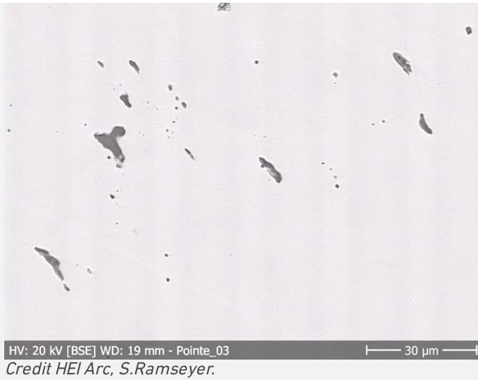
Fig. 6: SEM, BSE-mode picture of inclusions in remaining metal (detail of Fig. 5),
