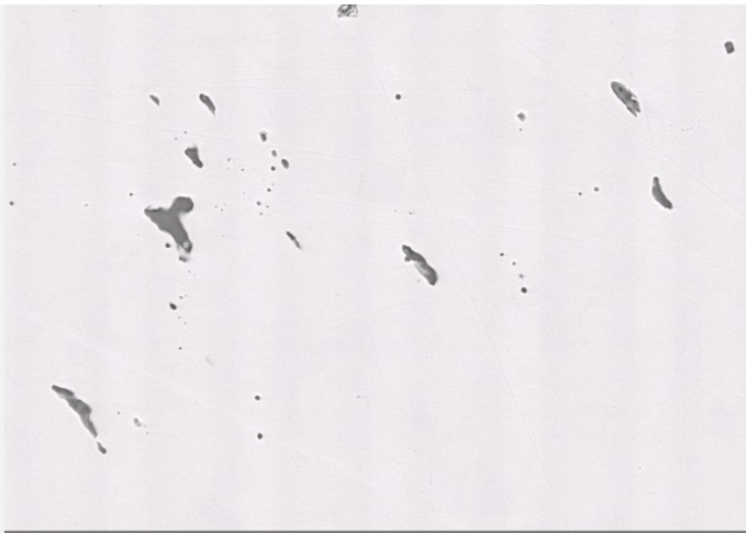
Fig. 6: SEM, BSE-mode picture of inclusions in remaining metal (detail of Fig. 5),
