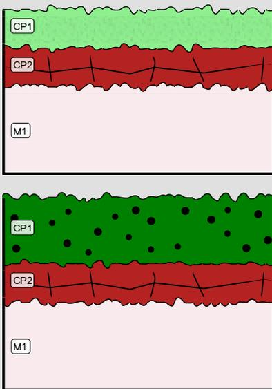
Fig. 9: Stratigraphic representation of the axe (sample 3) under binocular using the MiCorr application. The characteristics of the strata are only accessible by clicking on the drawing that redirects you to the search tool by stratigraphy representation. This presentation can be compared to Fig. 18. CP1 corresponds to CP1c, Credit HE-Arc CR, C.Degrigny.
