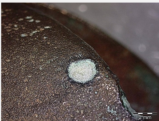
Fig 4: Local corrosion (diameter: 2 mm) where sample 1 has been taken,
