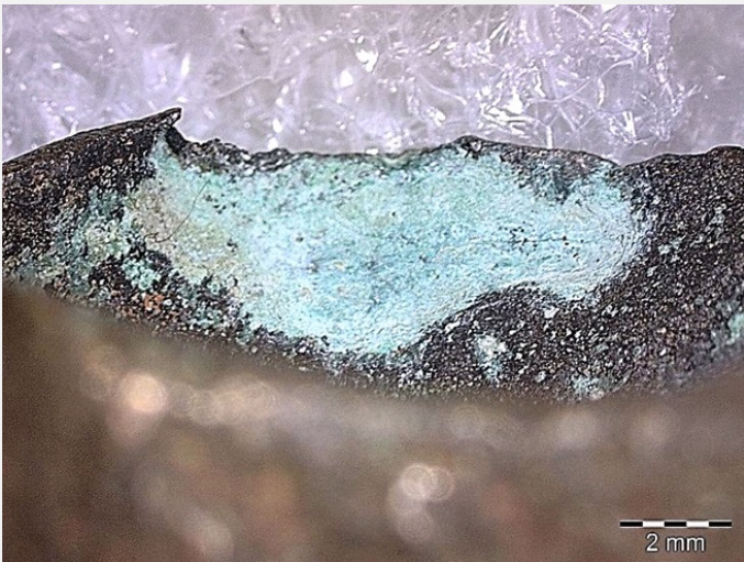
Fig. 6: Local corrosion (length max: 10 mm) where sample 3 has been taken,
