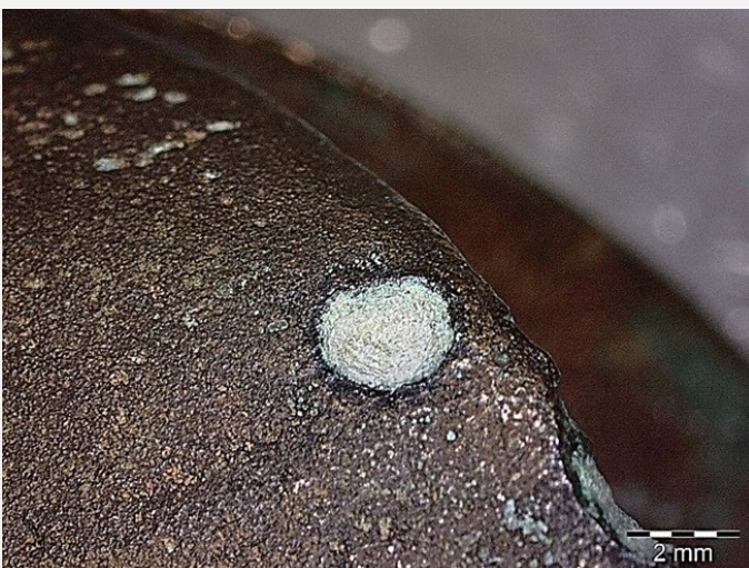
Fig. 4: Local corrosion (diameter: 2 mm) where sample 1 has been taken,
