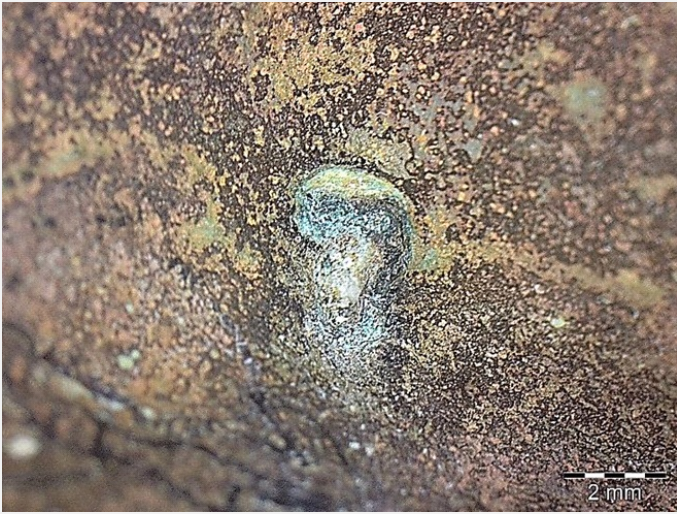
Fig. 5: Local corrosion (length max: 30 mm) where sample 2 has been taken,
