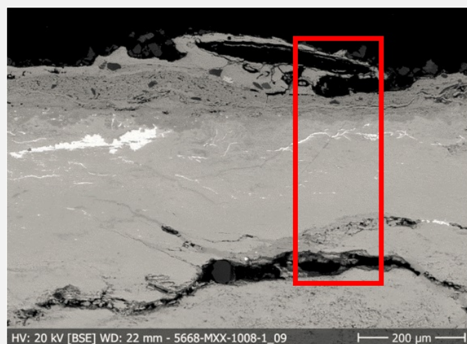
Fig. 9: SEM image of the cross-section from Fig. 8 (detail), BSE-mode. The area selected for elemental chemical distribution (Fig. 10) is marked by a rectangle,
