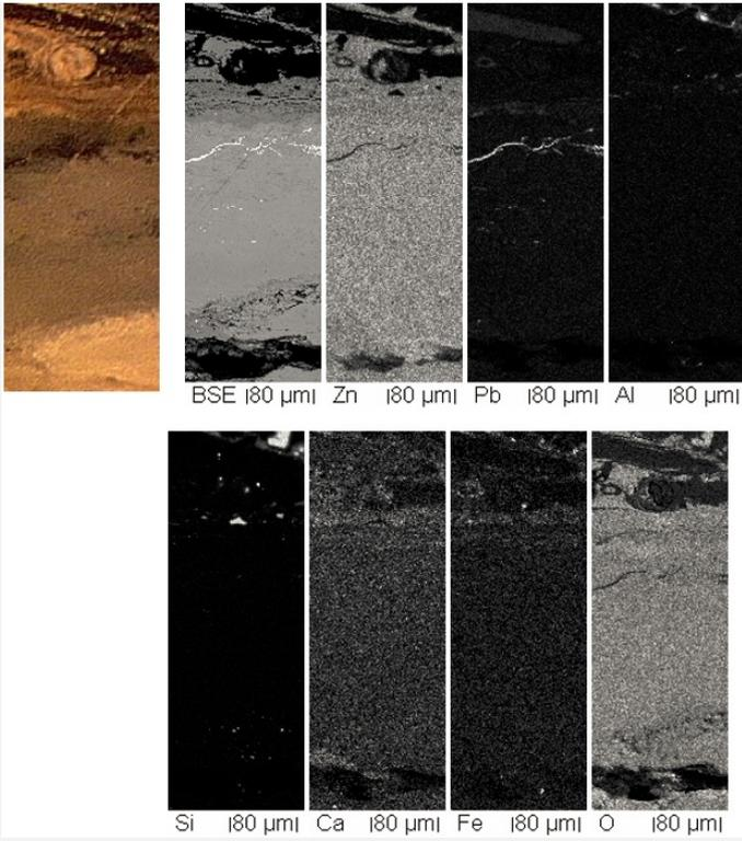
Fig. 10: SEM image of the cross-section from Fig. 9 (detail), SE-mode, and elemental chemical distribution. Method of examination: SEM/EDS, Lab of Electronic Microscopy and microanalysis, IMA (Néode), HEI Arc,
