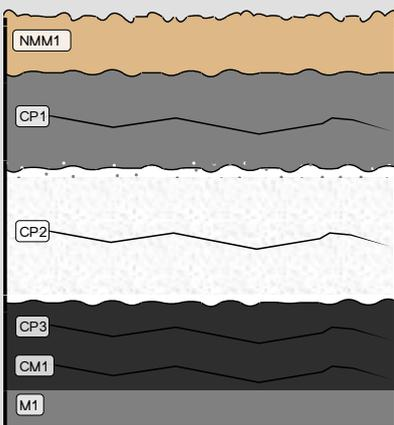
Fig. 16: Stratigraphic representation of fragment b of the military tag in cross-section (dark field) using the MiCorr application. The characteristics of the strata are only accessible by clicking on the drawing that redirects you to the search tool by stratigraphy representation. This representation can be compared to Fig. 10, Credit HE-Arc CR, M-J.Scholl.
