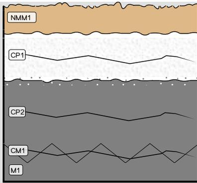
Fig. 17: Stratigraphic representation of fragment b of the military tag in cross-section (dark field) using the MiCorr application. The characteristics of the strata are only accessible by clicking on the drawing that redirects you to the search tool by stratigraphy representation. This representation is different from Fig. 10 due to the inversion of CP1 and CP2. Furthermore, CP3 is not represented, Credit HE-Arc CR, M-J.Scholl.
