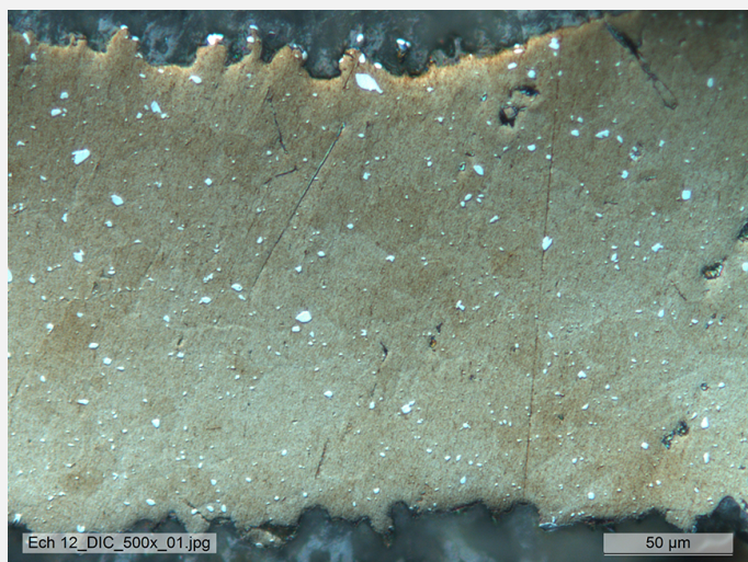
Fig. 7: Micrograph (detail of Fig. 5), unetched, dark field,
