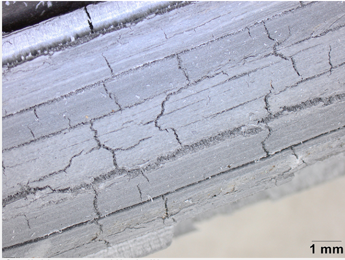
Fig. 3: Detail of the corroded lead came,
