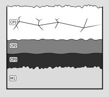
Fig. 4: Stratigraphic representation of the lead came under binocular using the MiCorr application. The characteristics of the strata are only accessible by clicking on the drawing that redirects you to the search tool by stratigraphy representation, Credit HE-Arc CR, A.Gerber.
