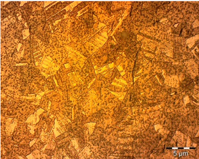
Fig. 6: Micrograph of the metal sample from Fig. 4, etched, bright field, 50x. Polygonal and twinned grains with strain lines are observed. The dotted surface is the result of over-etching,
