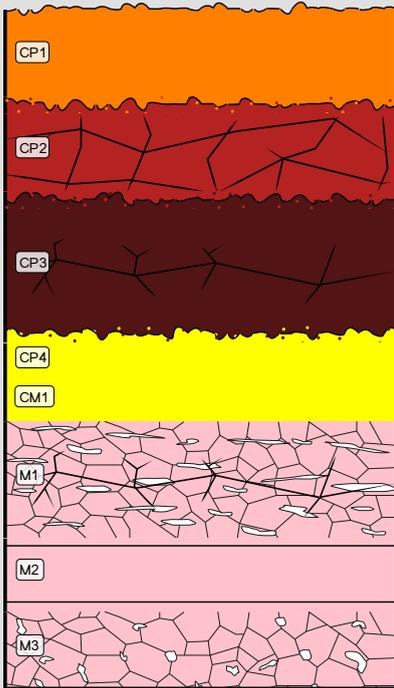
Fig. 14: Stratigraphic representation of sample 2 from the moil chisel in cross-section (dark field) using the MiCorr application. The characteristics of the strata are only accessible by clicking on the drawing that redirects you to the search tool by stratigraphy representation. This representation can be compared to Fig. 11, Credit HE-Arc CR.
