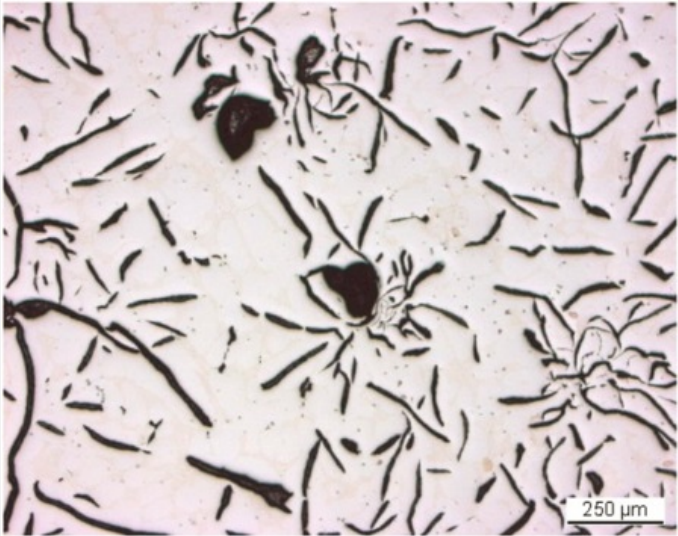
Fig. 4: Micrograph of the metal sample from Fig. 3 (inverted picture, detail), unetched, bright field. We observe graphite flakes and irregular nodules in black and the metal in white. The small grey spots are manganese sulphide inclusions,
