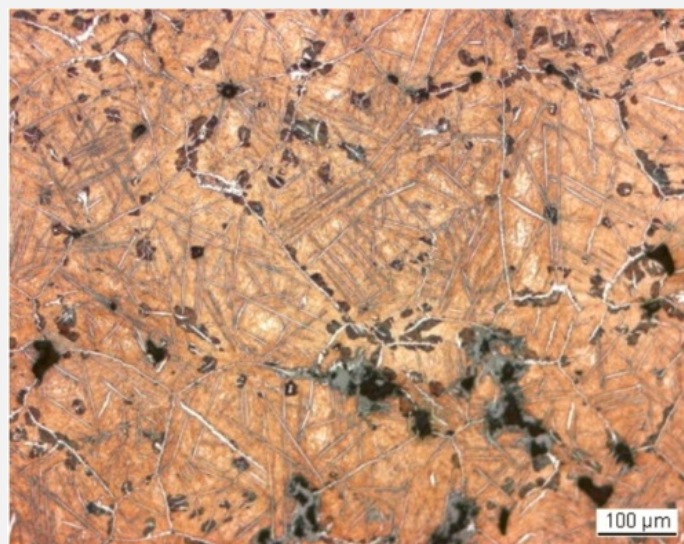
Fig. 8: Micrograph of the metal sample, detail from Fig. 4, etched, bright field. Hypereutectoid steel with a structure of cementite in white in the grain boundaries and in needle form combined with martensite (pink). Some bainite occurs around the grain boundaries,
