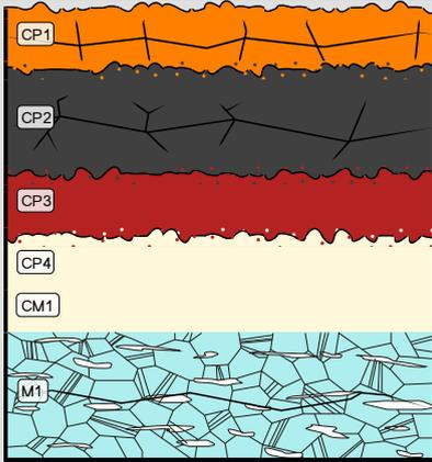
Fig. 10: Stratigraphic representation of the sample taken from the sword in cross-section (dark field) using the MiCorr application. The characteristics of the strata are only accessible by clicking on the drawing that redirects you to the search tool by stratigraphy representation. This representation can be compared to Fig. 8, Credit HE-Arc CR.
