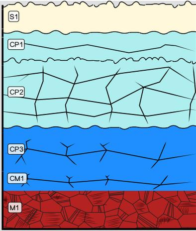
Fig. 14: Stratigraphic representation of the sample taken from the detached fragment of the situla in cross-section (dark field) using the MiCorr application. The characteristics of the strata are only accessible by clicking on the drawing that redirects you to the search tool by stratigraphy representation. This representation shows the interior face and can be compared to Fig. 8 (bottom red rectangle), Credit HE-Arc CR, M-J.Scholl.
