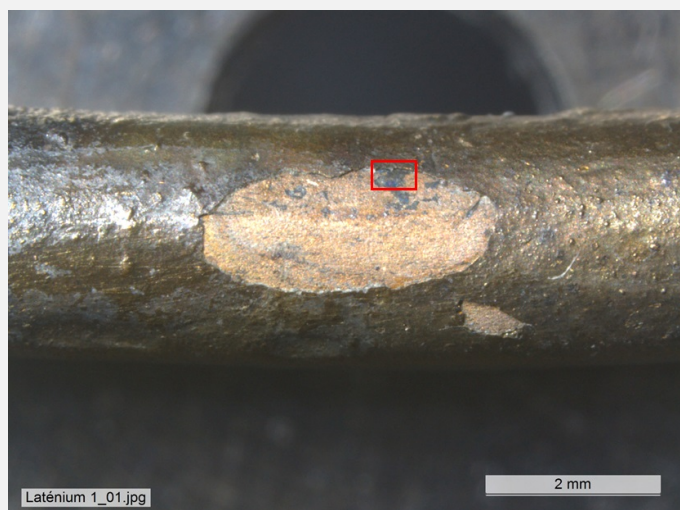
Fig. 2: Dense and smooth brown-yellow patina (detail) of the pin with lacuna showing the underlying metal with location of Fig. 4 (red rectangle),
