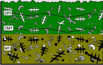
Fig. 11: Stratigraphic representation of the sample taken from the blade fragment of the winged axe in cross-section (dark field) using the MiCorr application. The characteristics of the strata are only accessible by clicking on the drawing that redirects you to the search tool by stratigraphy representation. This representation can be compared to Fig. 7, Credit HE-Arc CR.
