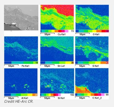
Fig. 9: SEM image, SE-mode, and elemental chemical distribution of a selected area of Fig. 4. Method of examination: SEM/EDS, Laboratory of Analytical Chemistry, Empa,
