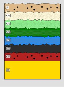
Fig. 3: Stratigraphic representation of the pin or needle fragment with green-blue patina under binocular using the MiCorr application. The characteristics of the strata are only accessible by clicking on the drawing that redirects you to the search tool by stratigraphy representation, Credit HE-Arc CR.
