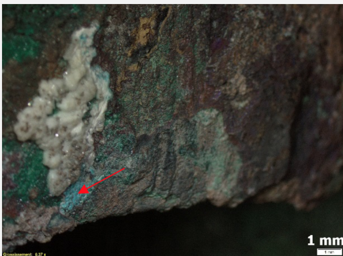
Fig. 17: Observation of the light blue corrosion product,
