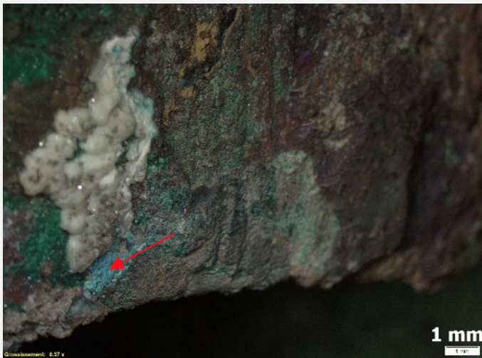
Fig. 17: Observation of the light blue corrosion product,
