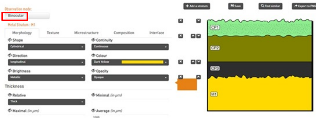
Digital stratigraphy of the corrosion structure observed under binocular.
